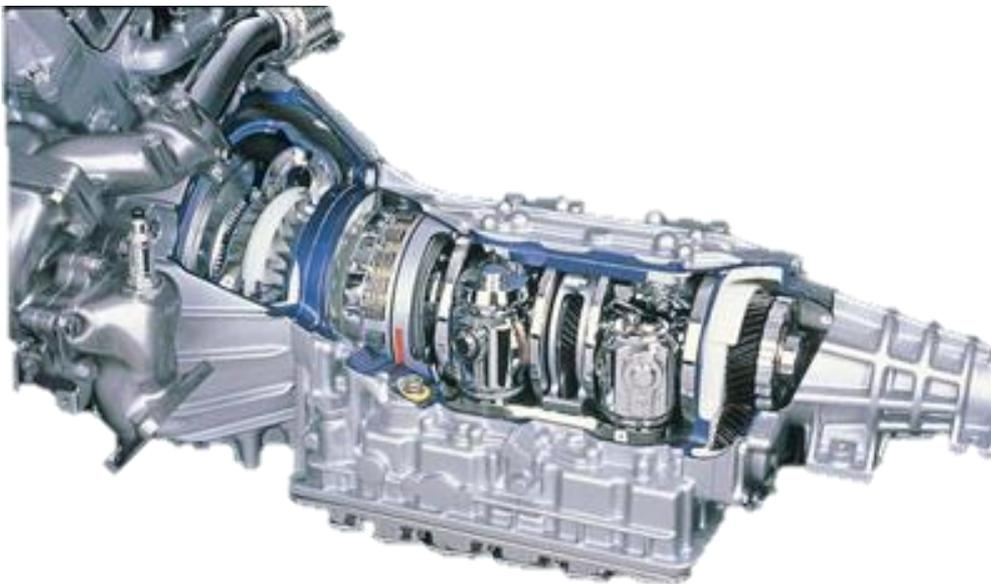
**Figure 7 Nissan Extroid toroidal CVT**
