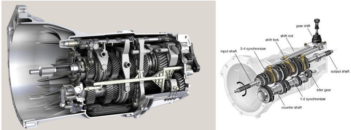
**Figure 1 ZF 6 speed manual transmission together with a manual transmission schematic.**
